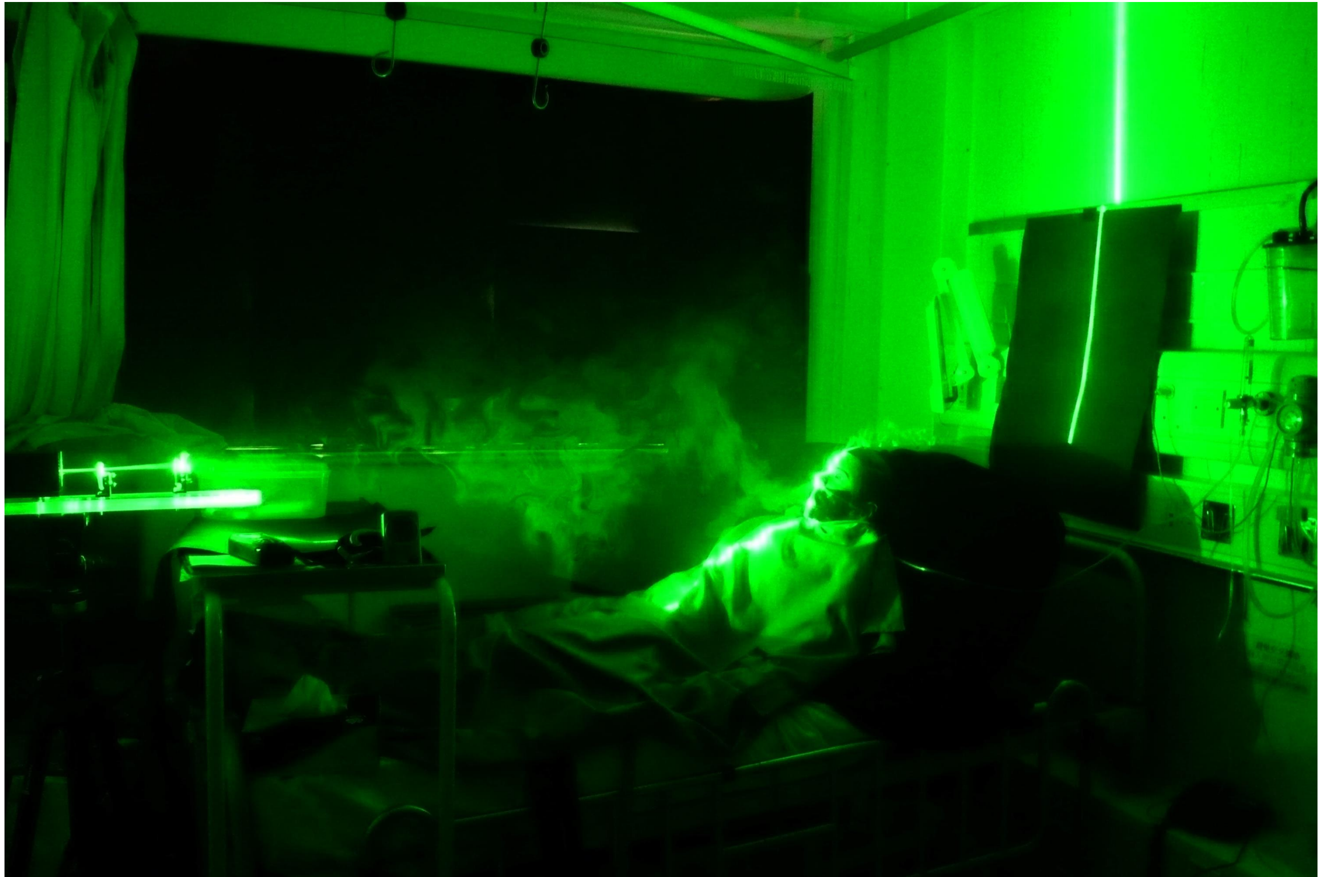
Figure: Experimental set-up, light sheet in sagittal plane at room B.
