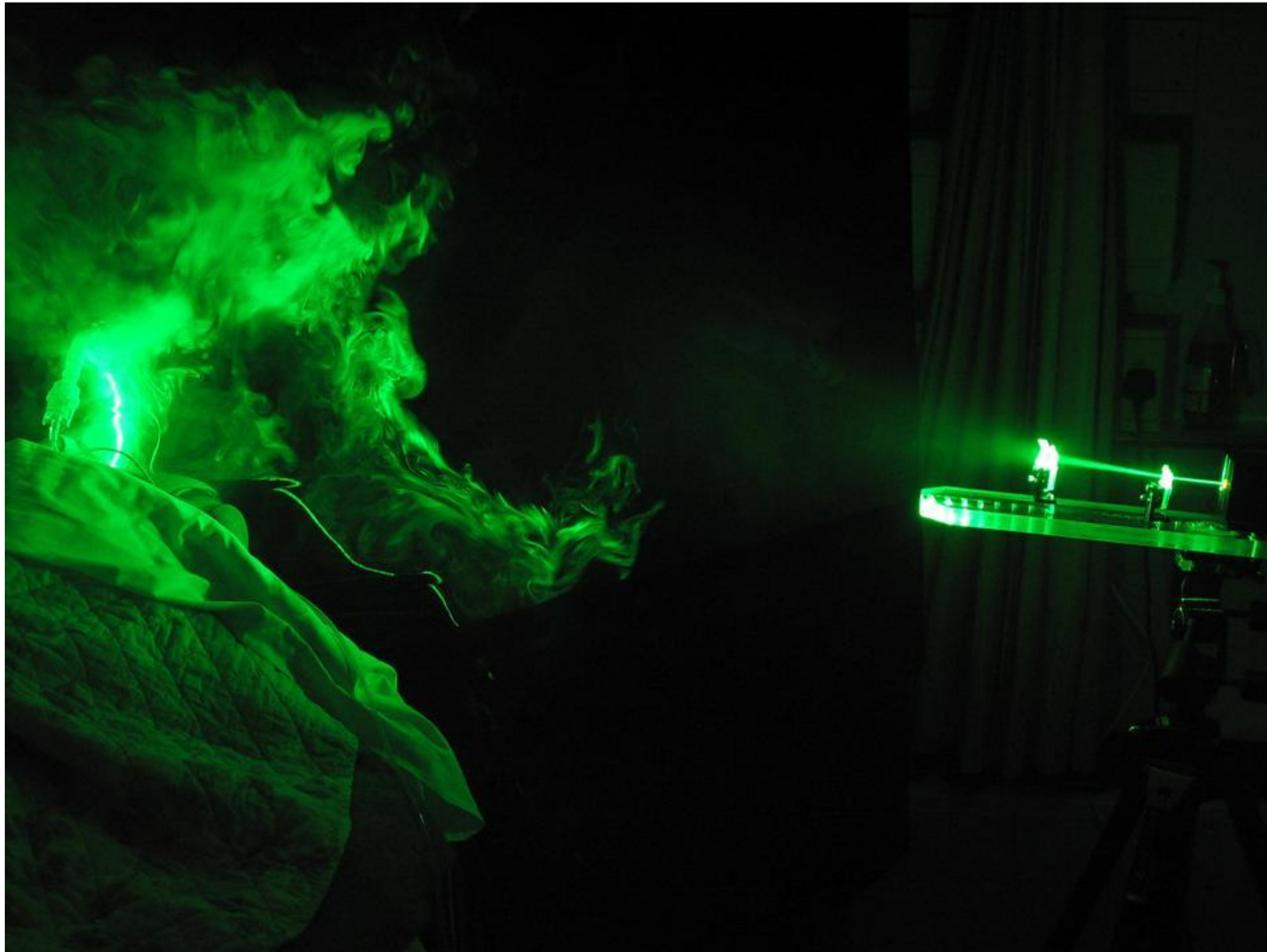
Figure: Photograph showing aerosol dispersion and patient exhaled air plume of jet nebulizer. Dr. Benny CHOW (ASHRAE-HKC/Med.CUHK)
