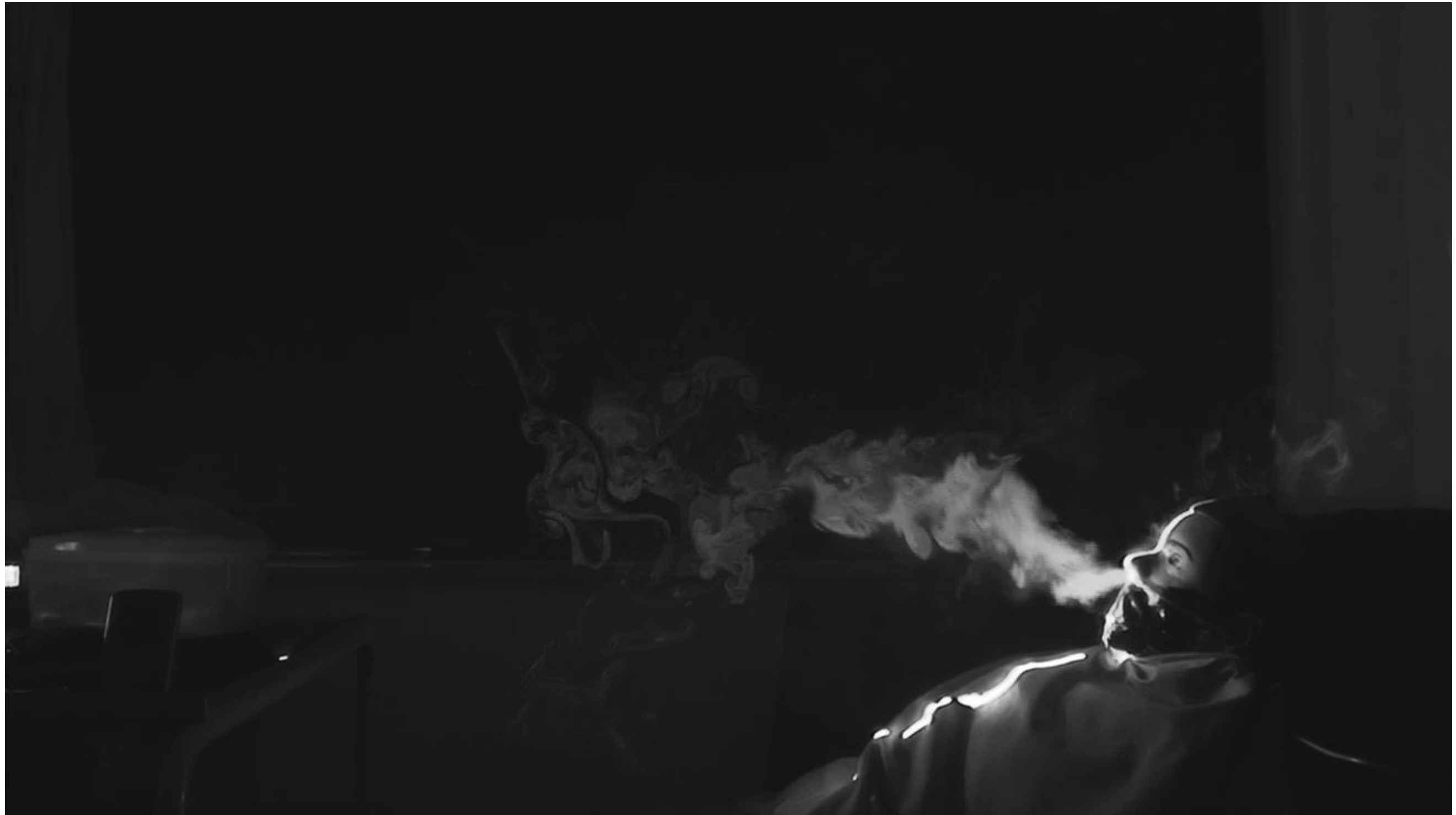
Figure: Grey scale camera frames captured for light intensity analysis routine to generate normalized particle concentration contours.
