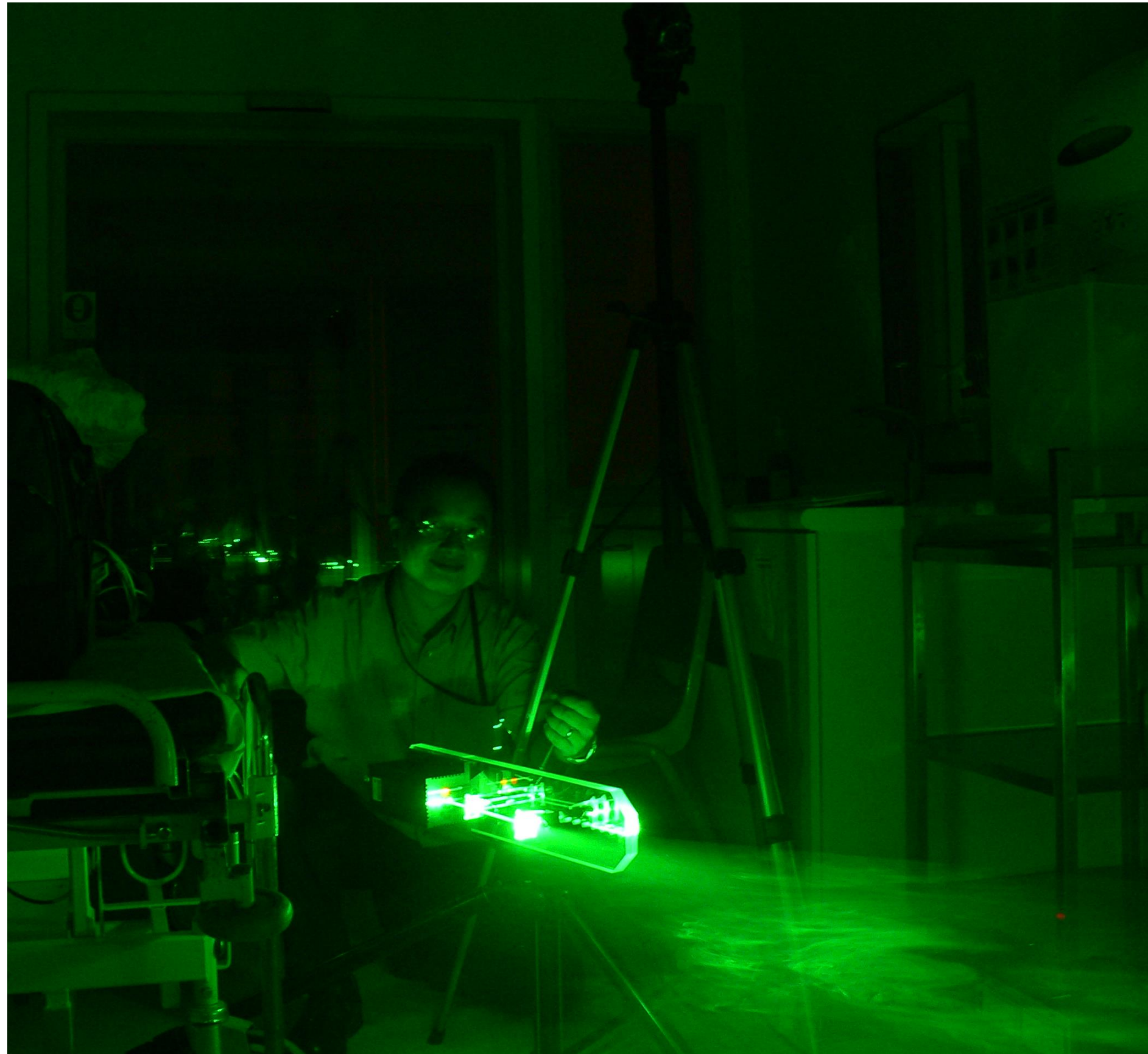
Figure: Laser flow visualization showing air enters in from the anteroom (right) to the patient room (left) from the door gap at the auto-swing door, (above) visual image (below) false color map of normalized smoke particle concentration.
