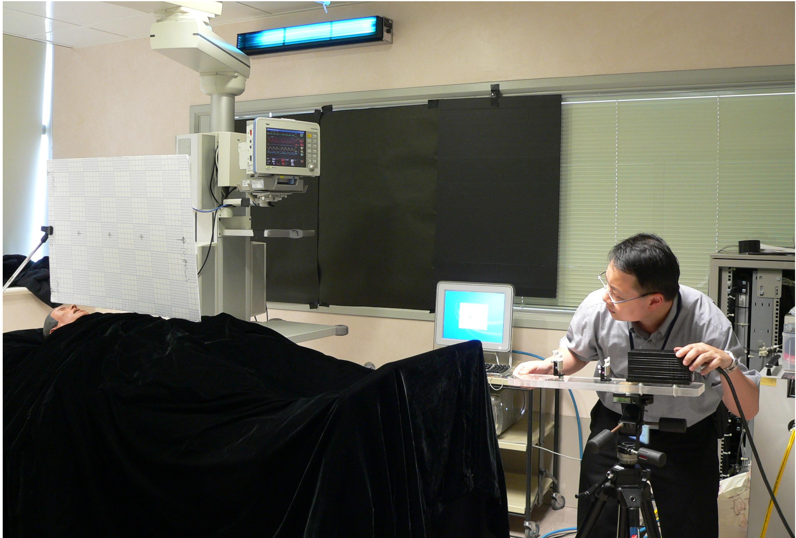
Figure: Calibrating the low-powered LIS with the dimension grid mounted on the median sagittal plane of the mannequin.
