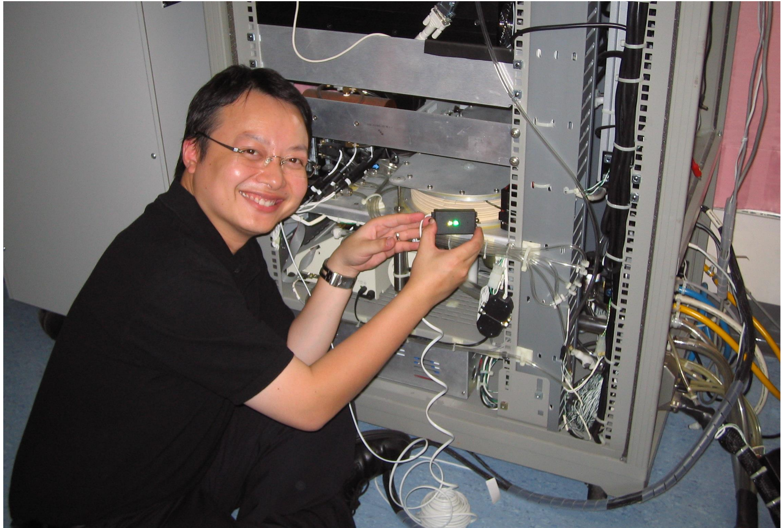
Figure: A mini device developed for the study to synchronize the mechanical movement of the HPS bellows with the laser imaging system (LIS).
