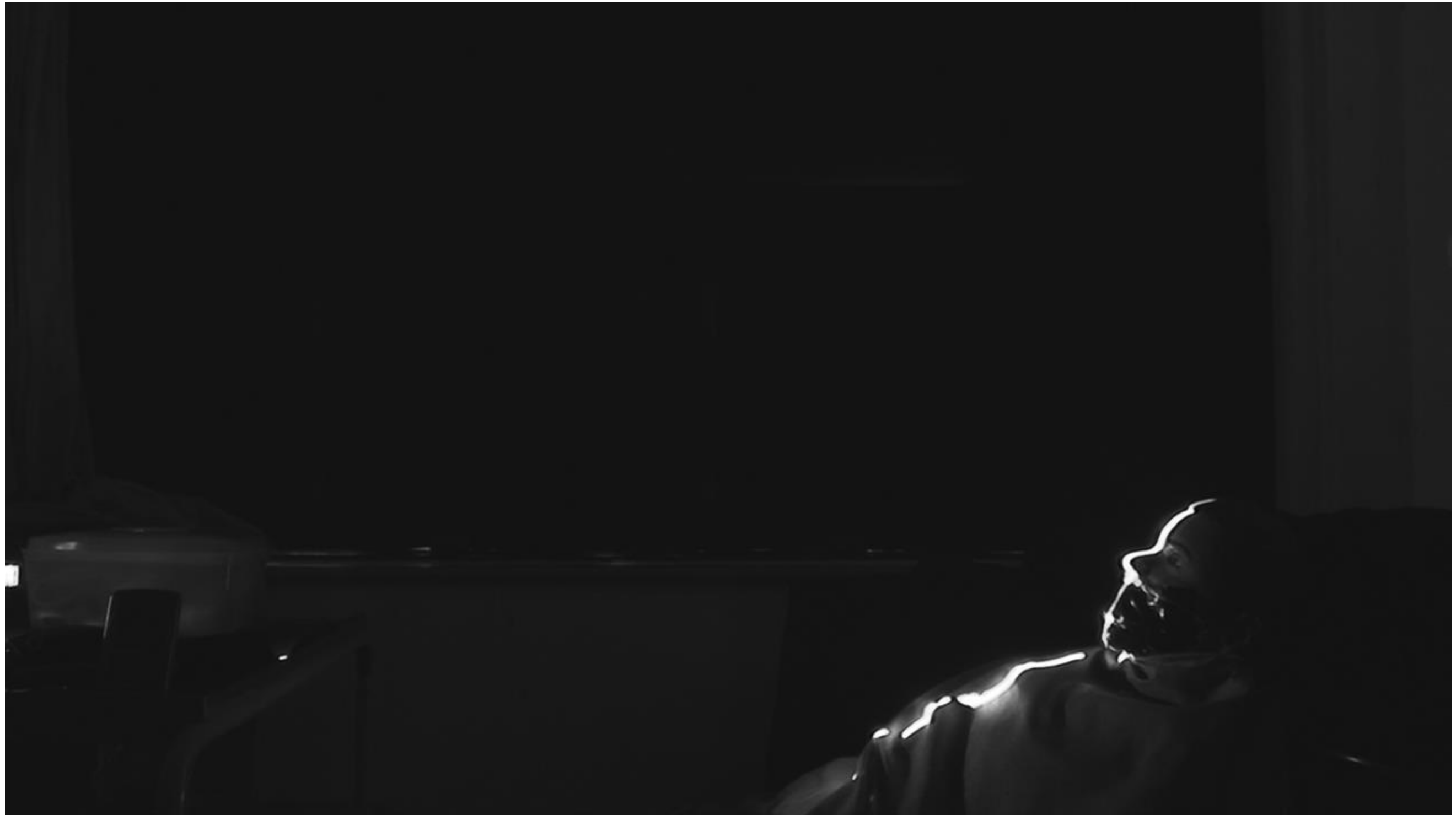
Figure: Background intensity image with ambient lighting switched off for stray background light subtraction.
