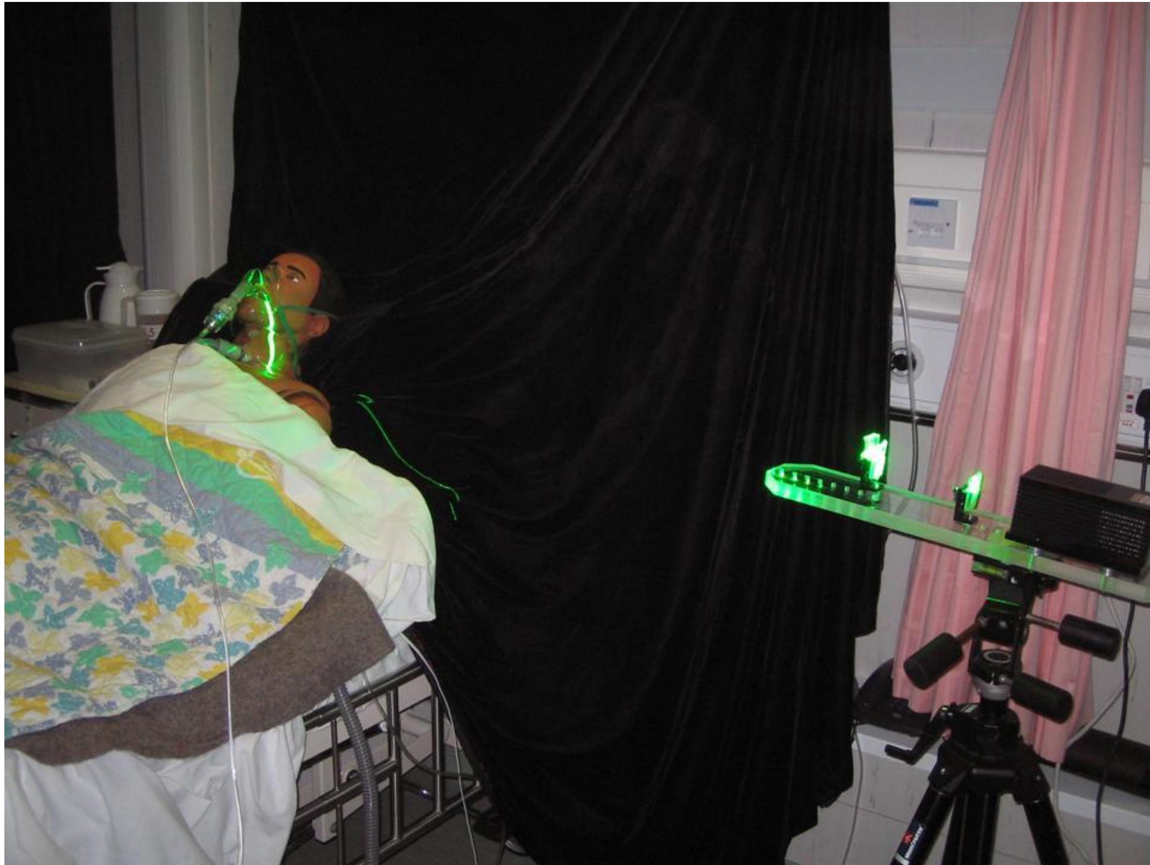
Figure: A jet nebulizer was attached to a HPS with a LST laser light sheet in the transverse plane.
